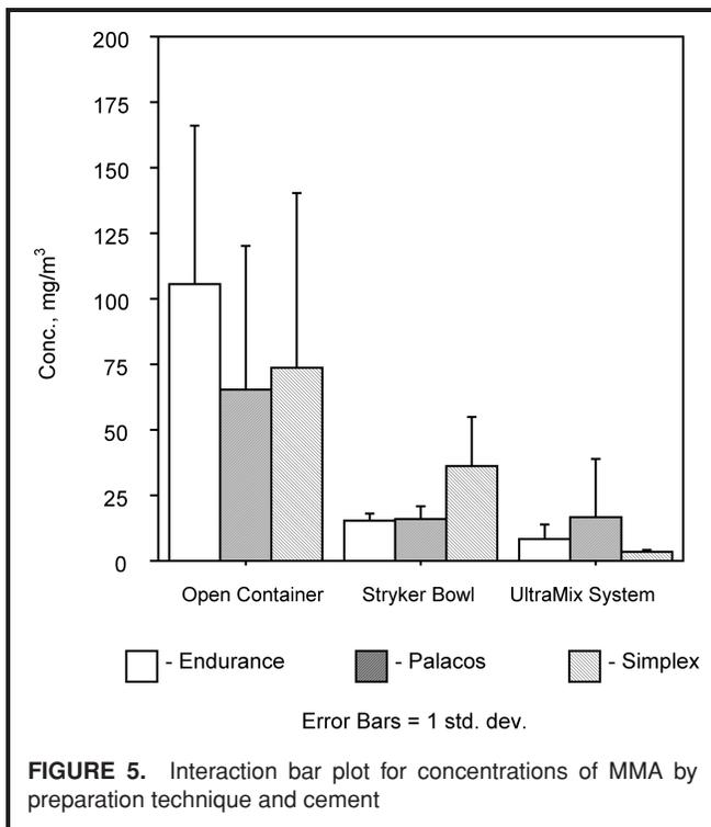
**FIGURE 5.** Interaction bar plot for concentrations of MMA by preparation technique and cement
