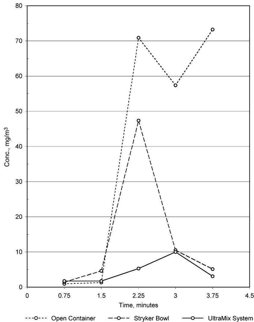
FIGURE 2. Emission-time profiles of mean MMA concentrations
